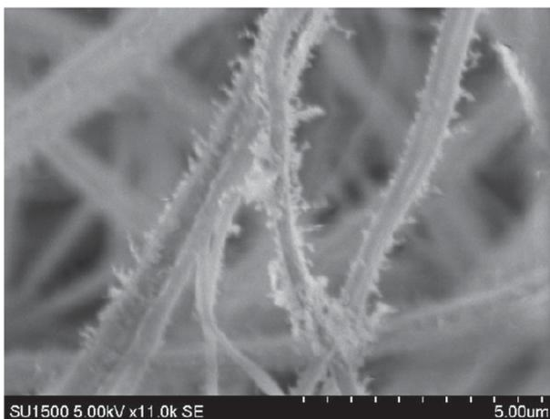
**Figure 8.** This graph shows hair-like or pearl chain-like structures over the fibres – the cause for reduced differential pressure.
