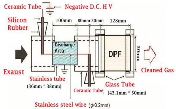
**Figure 2.** A modified system of an electrostatic precipitator and a diesel particulate filter.
