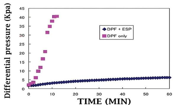
**Figure 5.** Exhaust back pressure increases abruptly with the installation of particulate filter only.
