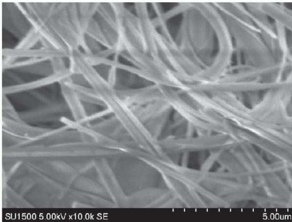
**Figure 6.** Clean fibres before the test fitting in the exhaust system.
