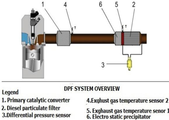
**Figure 1.** The overview of the modified system where an electrostatic precipitator is placed before a diesel particulate filter.
