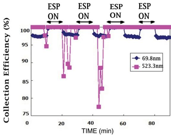
**Figure 3.** Collection efficiency increases up to 99.9% when the electrostatic precipitator is powered on.
