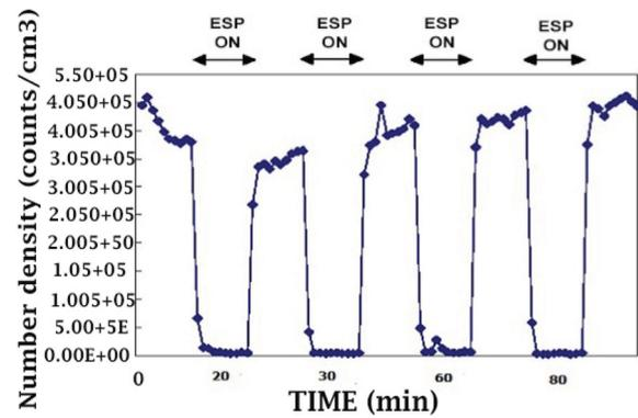
**Figure 4.** Graph showing the decrease in PM when the electrostatic precipitator is switched on.
