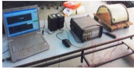
Fig. 5: Impact testing instrumentation set up
