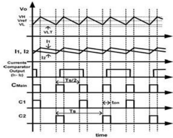
**Figure 4** General waveform samples for the current division method
