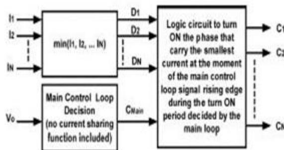
**Figure 2** Basic functional diagram of the Proposed Method
