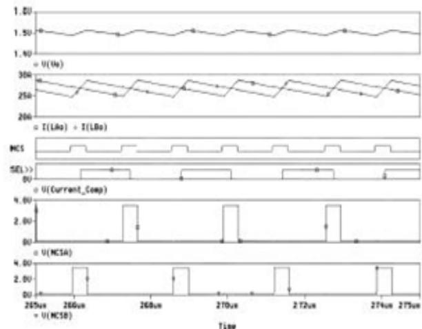
**Figure 9** Simulation outputs in logic 0 to Logic 1 Load Transient State
