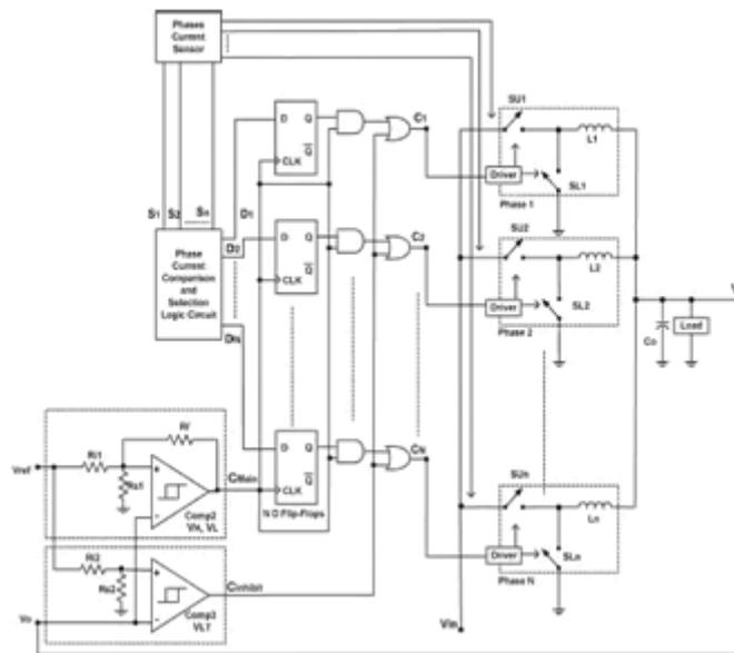
**Figure 5** Fundamental controller diagram of N multiples of voltage-mode (ripple) hysteretic strategic current sharing (division) converters.
