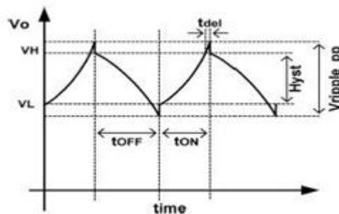
**Figure 6** Output Voltage with its Ripple and delay time
