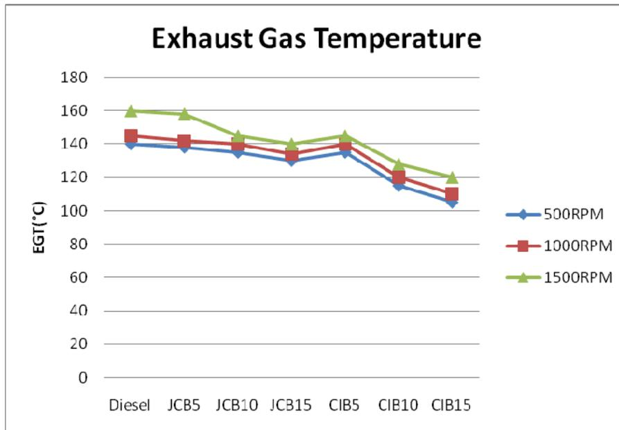
**Figure-4.** Exhaust gas temperature at multiple idling situations for diesel, Jatropha curcas biodiesel and Calophyllum biodiesel blend.
