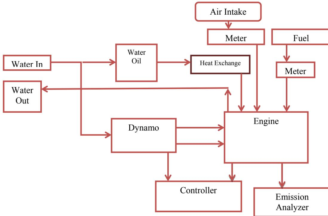
**Figure-1.** Schematic diagram of the engine test bed.
