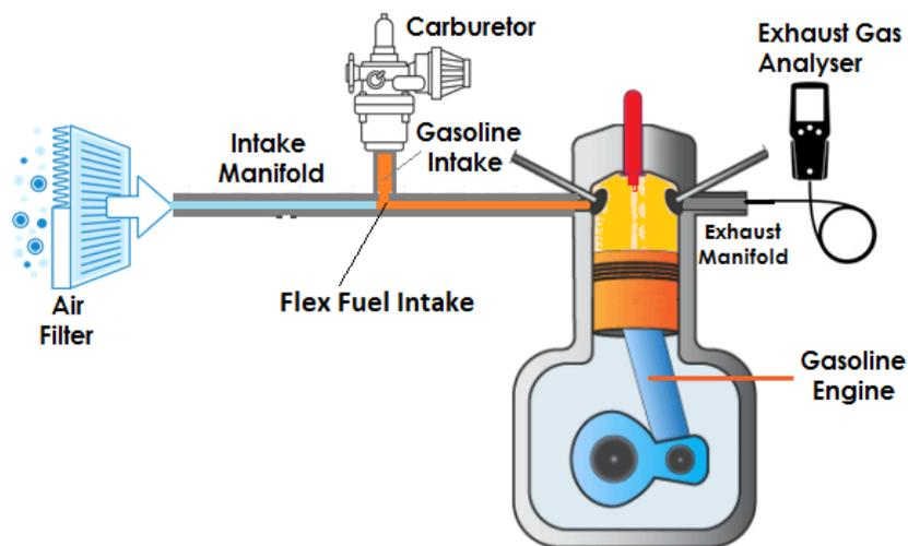
Fig. 1: Schematic diagram of the Flex Fuel setup.
