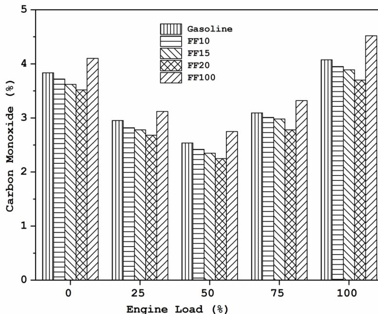
Fig. 4: Impact of flex fuel on carbon monoxide.
