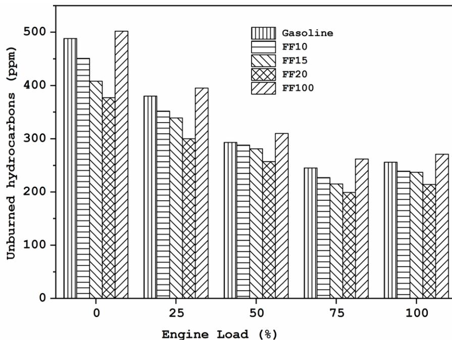
Fig. 5: Impact of flex fuel on unburned hydrocarbon.
