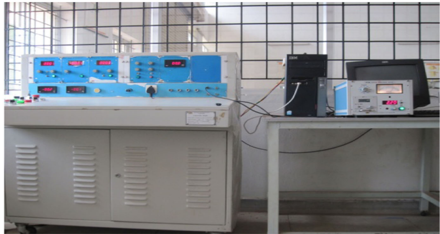
(a) Control Panel used to perform flashover test analysis.
