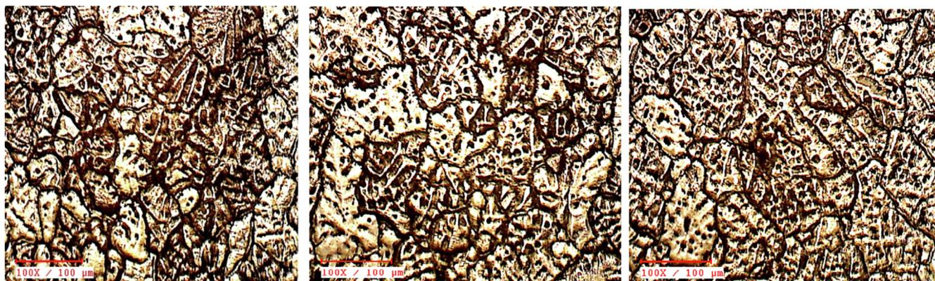
Fig. 2. Microstructures of Al7075 aluminium composites reinforced with TiC of varying weight percentage of 3, 6, and 9%
