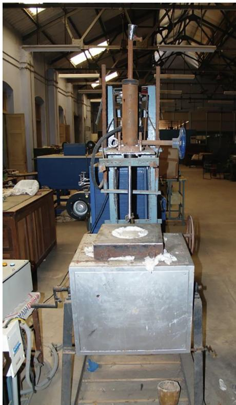
Fig 1. Stir casting setup.
