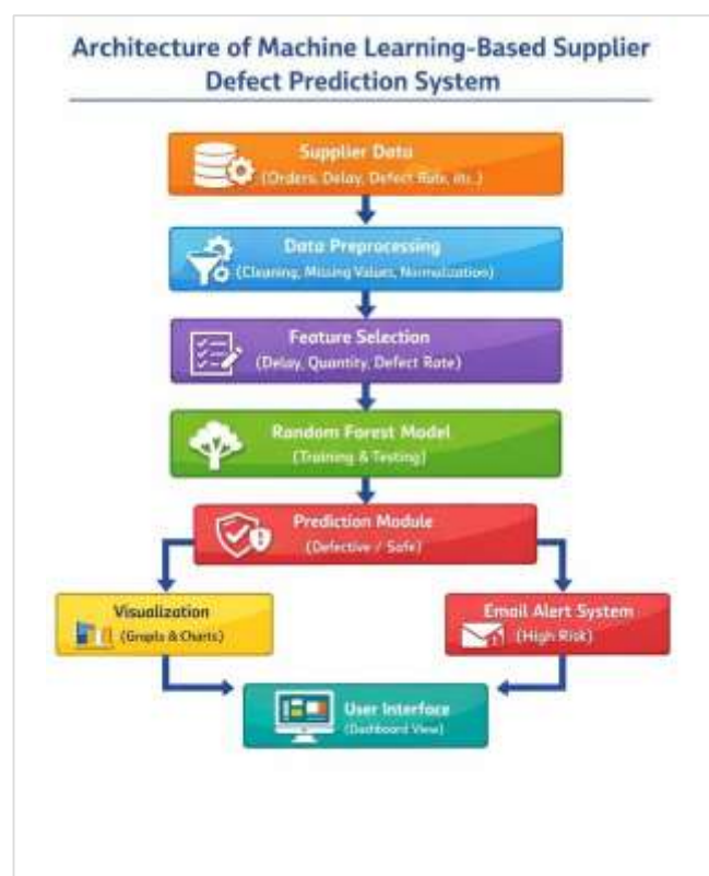
Fig. 1 Architecture of Machine Learning-Based Supplier Defect Prediction System
