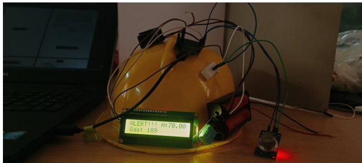
Prototype of the Miner's Safety Helmet when detecting hazardous gas and humidity.
