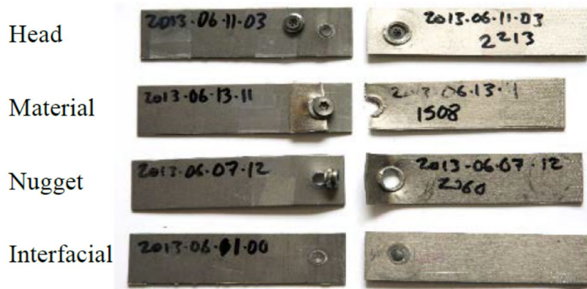
Figure 7. Four failure modes of FBJ joints (Peterson, 2015).
