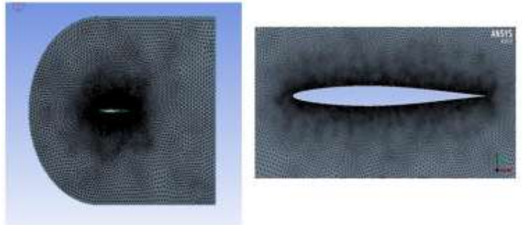
Figure No: Leading Edge Radius 5.2– 0 Degree
