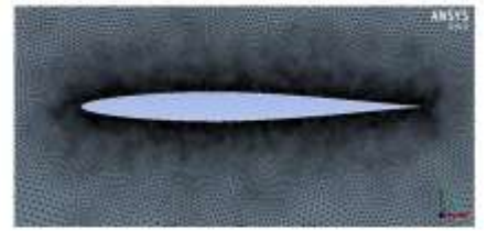
Figure : Leading Edge Radius 5 – 0 Degree AOA of NACA64008 aerofoil
