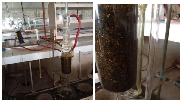
Figure 2: Soxhlet extraction set-up of Hybanthus enneaspermus 19,20
