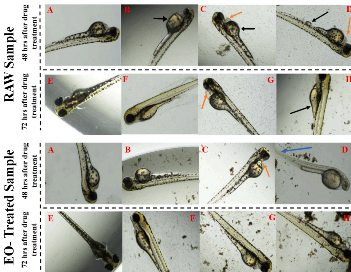
Fig. 7. Genotoxicological assessment of raw and treated hospital wastewater (HWW) using zebrafish embryos at 48 and 72 h post-fertilization (hpf). RAW Sample: Panels A–D: HWW at 48 hpf showing dose-dependent yolk sac edema, pericardial edema, reduced pigmentation, and tail deformities. Panels E–H: Raw HWW at 72 hpf showing aggravated malformations, including severe pericardial/yolk sac edema and axial defects. EO-treated Sample: Panels A–D (treated): HWW at 48 hpf showing largely normal development with only mild, transient abnormalities at higher doses. Panels E–H (treated): EO-treated HWW at 72 hpf showing normal morphology across all concentrations. Orange arrows: pericardial edema; Black arrows: yolk sac edema; Blue arrows: tail abnormalities. (For interpretation of the references to colour in this figure legend, the reader is referred to the web version of this article.)
