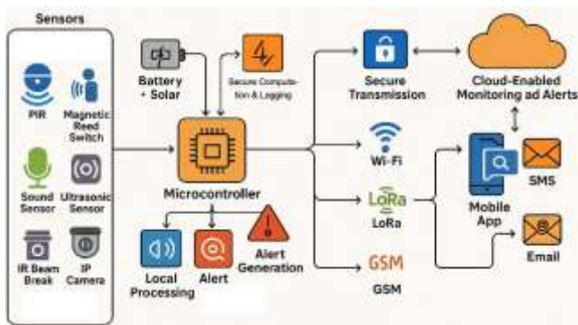
Fig 2. Architecture of the Proposed IoT-Enabled Residential Intrusion Detection System
