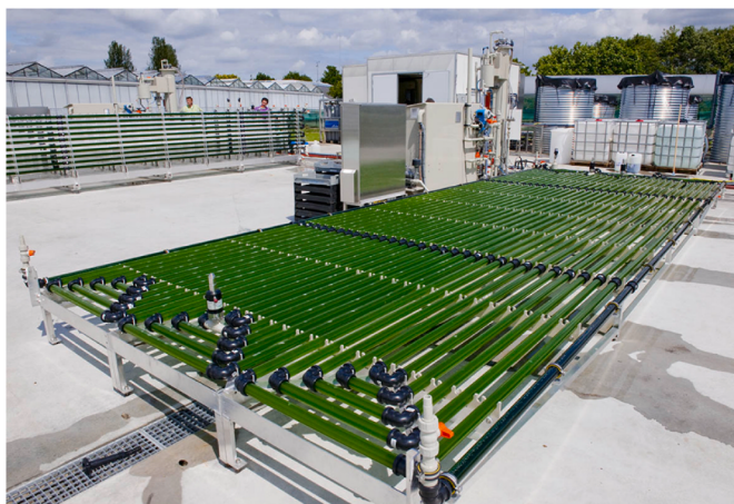
Fig. 4. A horizontal tubular algal photobioreactor set up at the Wageningen University, Netherlands (vertical tubular photobioreactor at top left) [148].
