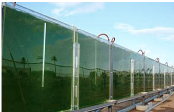
Fig. 5. A vertical flat plate photobioreactor set up at the Arizona Center for Algae Technology and Innovation, Arizona State University, USA (energy.gov).
