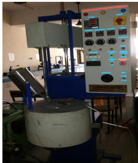
Figure 4. Aluminum stir caster setup
