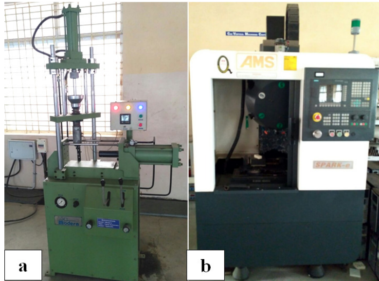
Figure 3 (a) Hydraulic Injection Moulding Machine (b) Vertical CNC Machine
