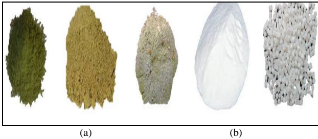
Fig. 1: Fabrication of NFRPC [a] to powder with polypropylene [b] particles
