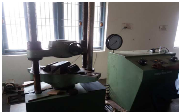
Figure 2: Experimental Set-Up to Obtain the Static Load-Displacement Curves
