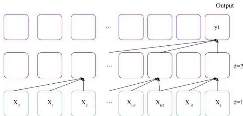
Fig. 4 Temporal Convolutional Network (TCN) architecture for time-series forecasting
