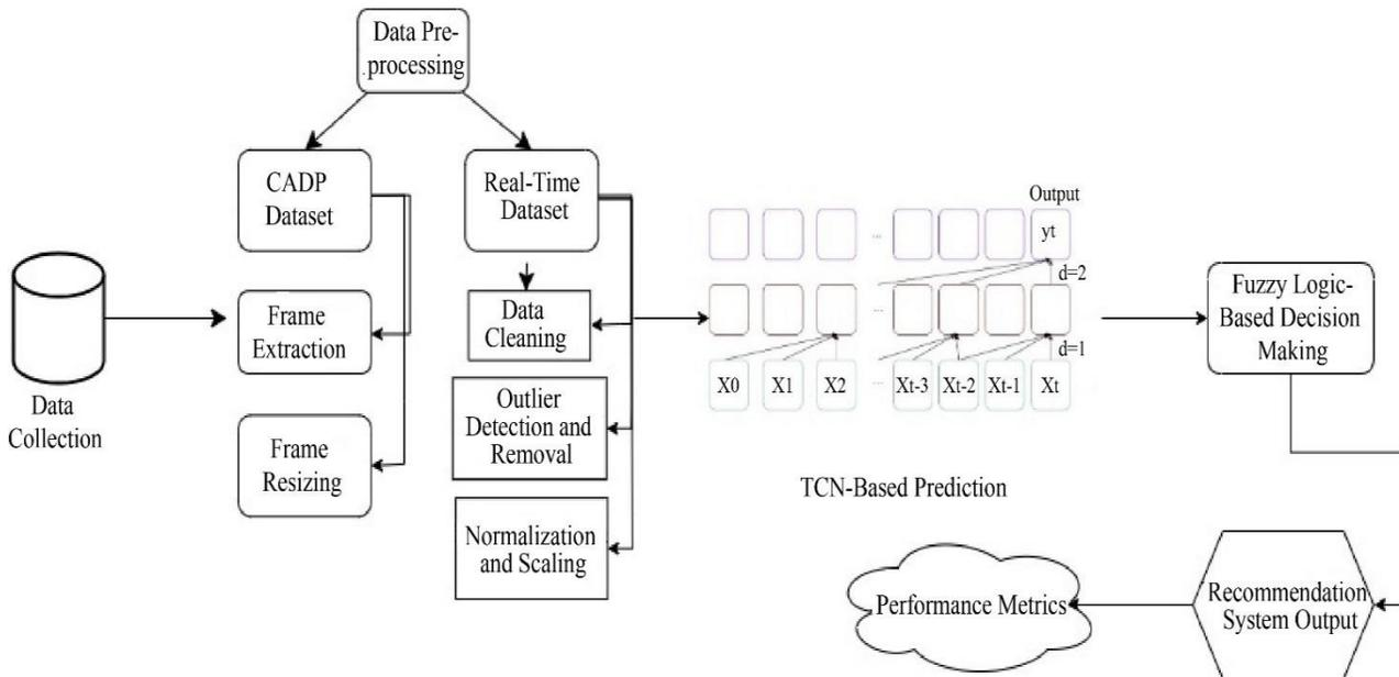
Fig. 1 Overall workflow of TCN-Fuzzy logic
