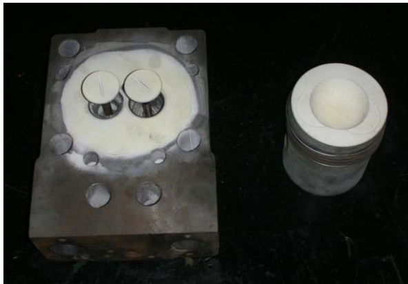
Figure-1. Thermal barrier coating on the piston crown, cylinder head and valves.
