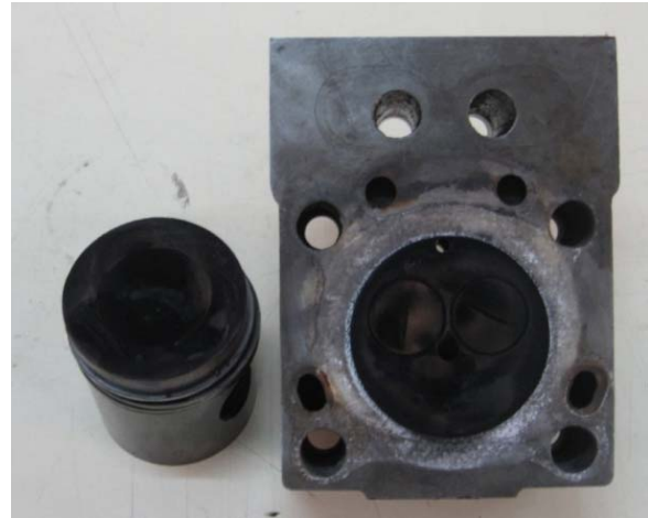
Figure-2. Soot formation on thermal barrier coating.
