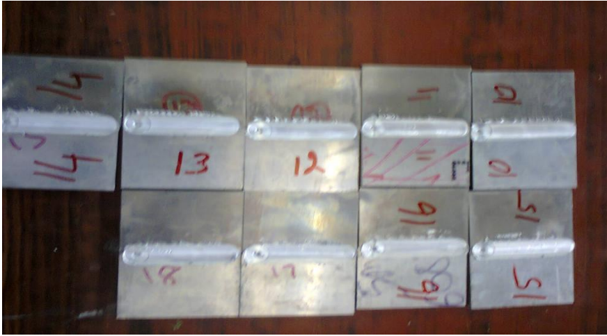
Fig. 2. After welded specimen
