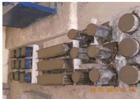
Figure 5. Fresh concrete specimens
