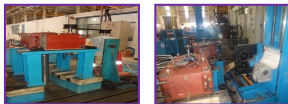
Figure 3. Before and after Vertical type gear box testing setup
