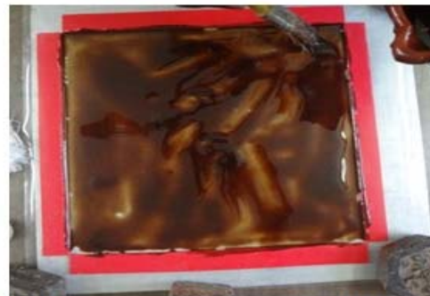
(c) Mould preparation with coconut shell powder
