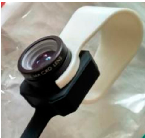
Figure 3. Magnification lens of power 20×.
