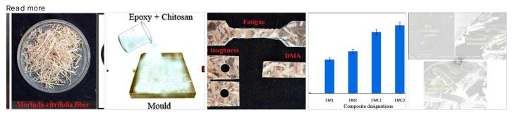
Tensile fatique, fracture toughness, and thermo-mechanical behavior of silane-modified Morinda citrifolia fiber and chitosan-reinforced epoxy composites
