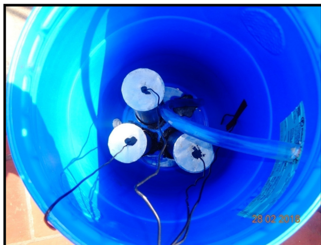
Fig. 4. PCM tank containing 3 PCM cylinders of 250 g each with 3 g of aluminium oxide.
