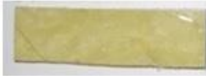
FIGURE 3. Sample Specimen of Hybrid Composite for Characterizing Properties under Orthogonal load
