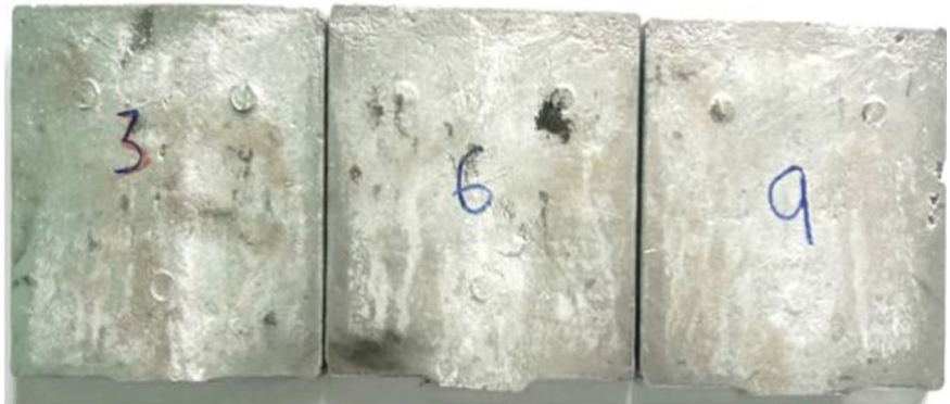
(b) Composites of silicon nitride obtained using squeeze casting by varying its weight percentage (3%, 6% & 9%)
