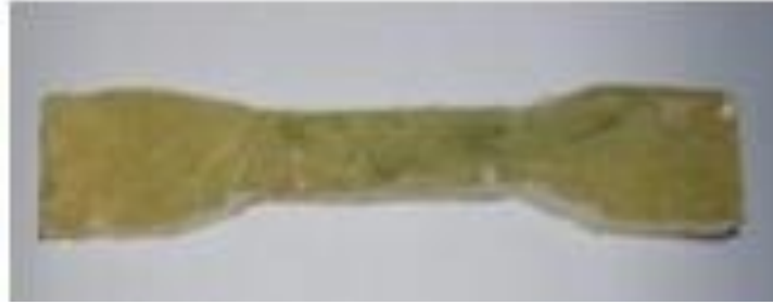
FIGURE 2. Sample Specimen of Hybrid Composite for Characterizing Properties under Co-linear unlike load
