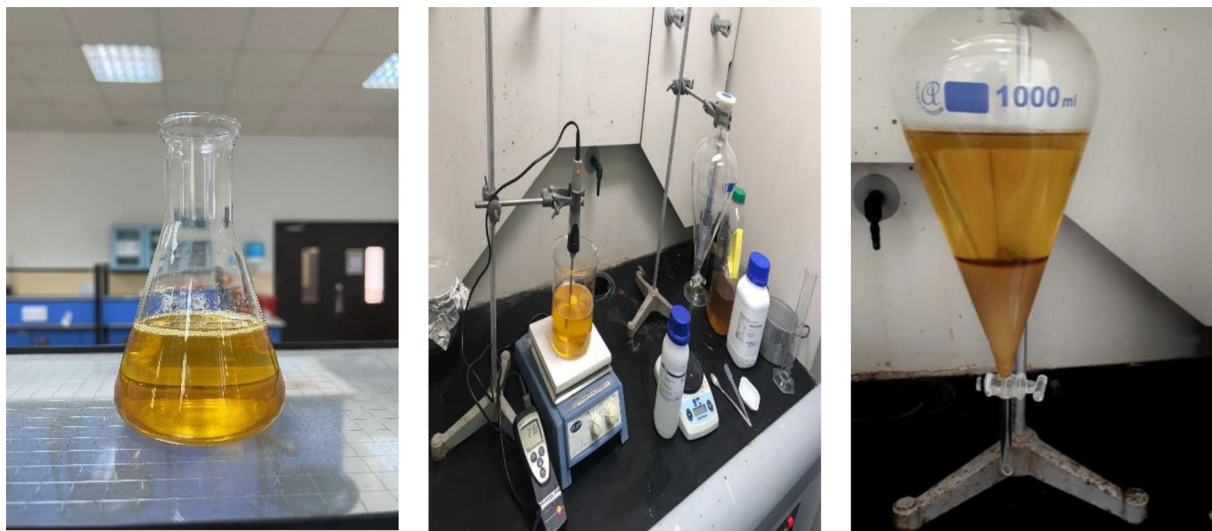
Figure 2. Experimental setup: (a) Mixed crude sunflower-mahua oil; (b) Experimental setup and (c) Biodiesel and glycerol in separating funnel.
