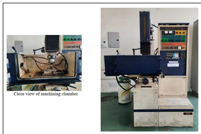
Fig. 7. Schematic diagram of the EDM machine (Courtesy: National Institute of Technical Teachers' Training and Research, Chandigarh, India).
