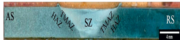
FIGURE 2: Microstructural welding zones of friction stir-welded aluminium alloy.
