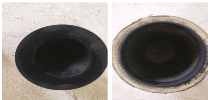
FIGURE 4: After 100 hours of operation, the piston and cylinder liner are coated.
