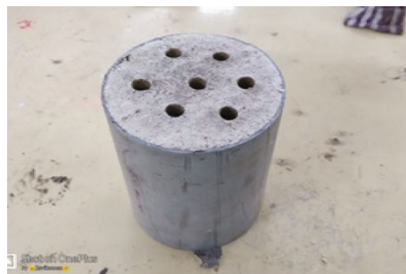
FIGURE 5: PVC pipes as mold cavity.
