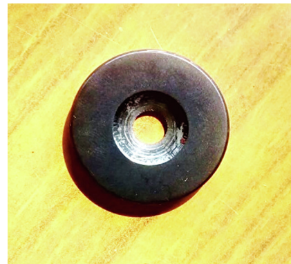
Fig. 12. Wear Test results on Coated Specimen After Wear Test.
