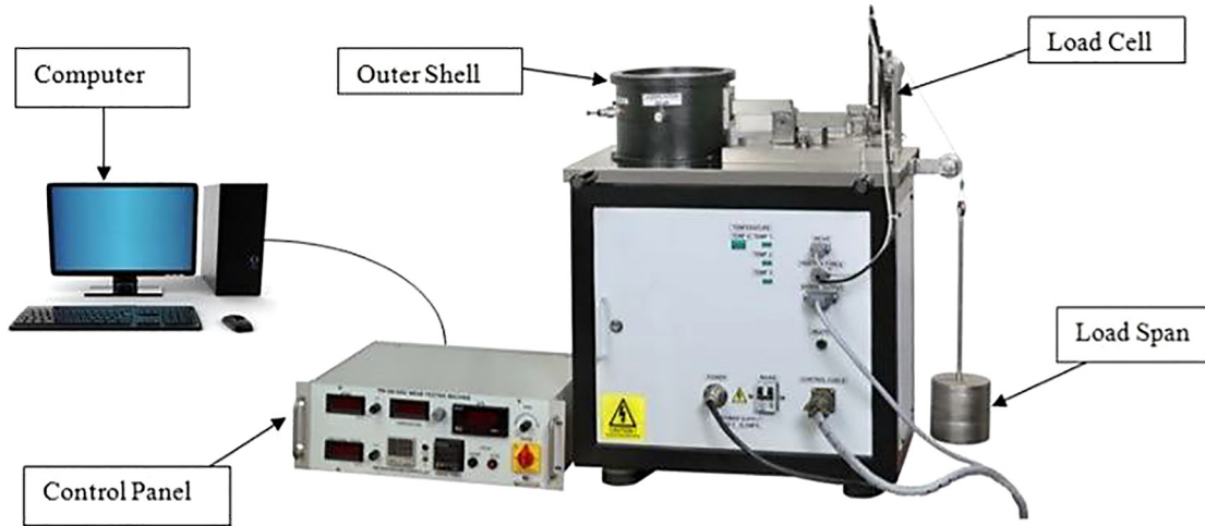
Fig. 4. Experimental arrangements of Pin On Disc [POD].
