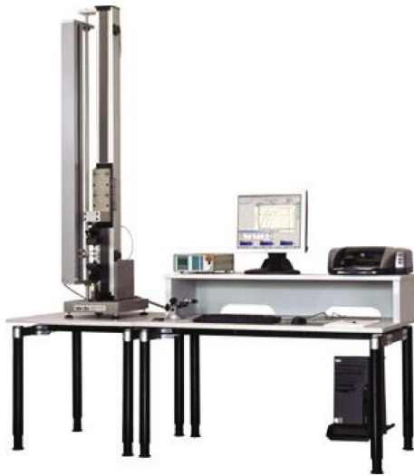
FIGURE 6: Multipurpose microtensile testing machine.
