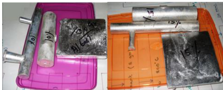
Fig. 4. A photographic view of AA 6061/SiC casted samples.
