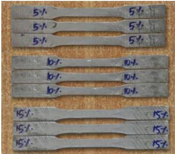
Fig. 9. AA 6061/SiC specimens for tensile test.
