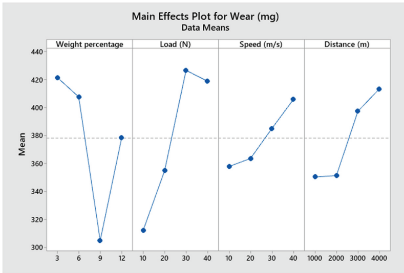
Figure 2. Wear rate of AA7168/SiC/B 4 C particulate reinforced hybrid composite.
