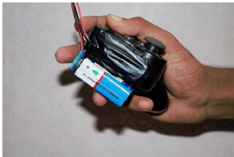
Fig. 10. Gesture – 3 moves the 2nd servo in reverse direction.
