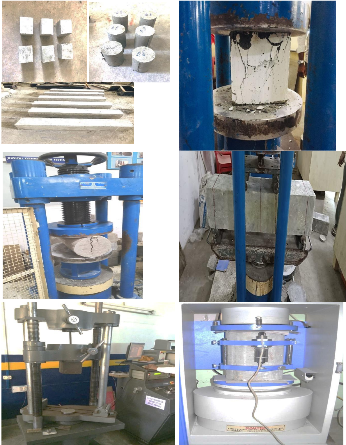
Figure 2. Test setup on Compressive strength, Split tensile strength, Flexural strength, Pull-out test and Modulus of Elasticity of concrete
